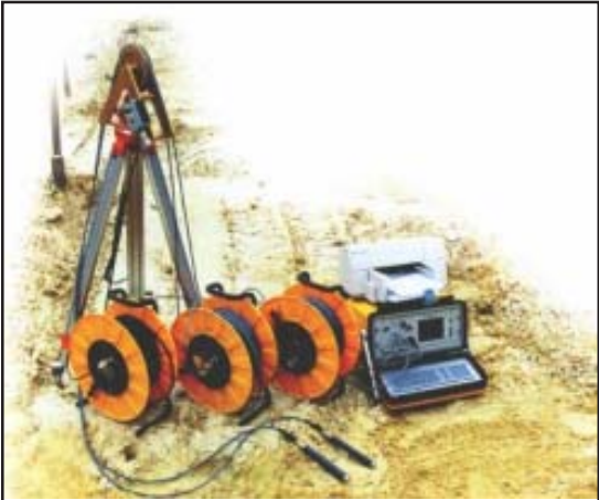
Fig. 2 Crosshole Sonic Logging CS 97 Apparatus
